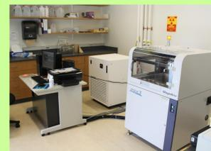
Samples were analyzed using a Rigaku ZSX-3 X-ray fluorescence instrument for major oxides (in weight percent) and trace elements (in parts per million, ppm).
